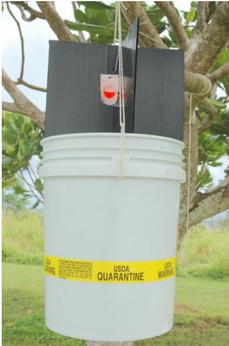
Figure 1: Coconut rhinoceros beetle pheromone trap. Made by the Agricultural Development Service, Guam Department of Agriculture
