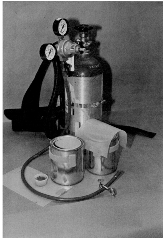
Fig. 1. Components of the lightweight baited trap showing can with Velcro, canopy, and bait cup containing aluminum screening over 2 g dry distiller's grain (left foreground), an assembled trap (right foreground), and a 2.3-kg tank of gaseous CO 2 fastened to a small Scuba backpack frame.
