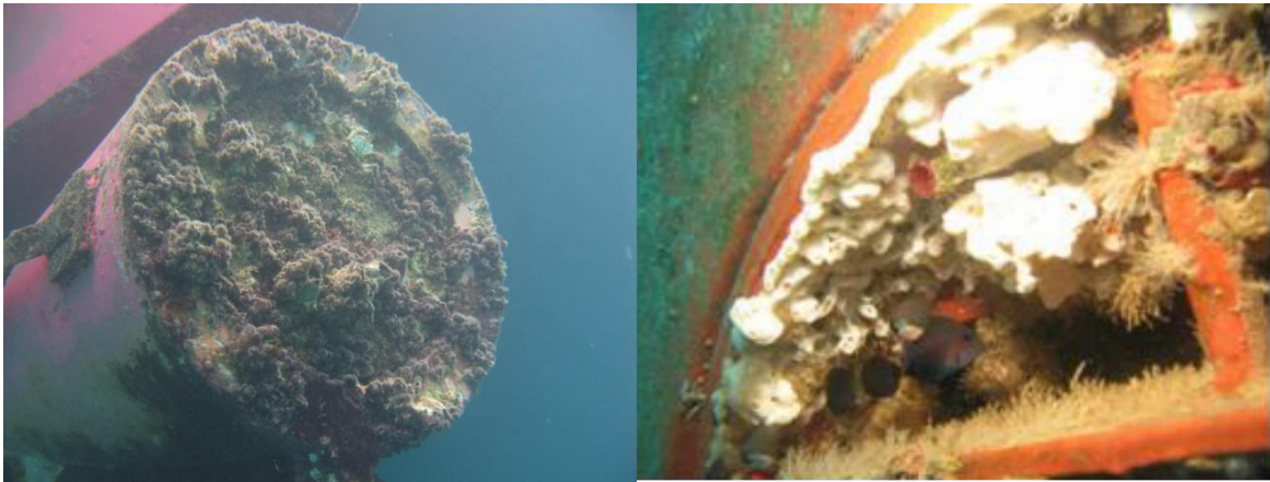
Figure 2.1. Biofouling organisms on vessels arriving to Guam. Left: High percent cover of fouling organisms below the rudder. Right: Sessile species such as sponges, tunicates and hydroids, growing on a grate provide habitat for mobile species.
